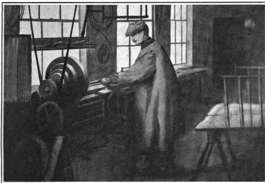
AN INTERESTING INCIDENT AT QUEENS — JOSEPH TRACY (NO. 3) TURNING UP A NEW PIN FOR PROPELLER SHAFT JOINT IN A WAGON SHOP.
